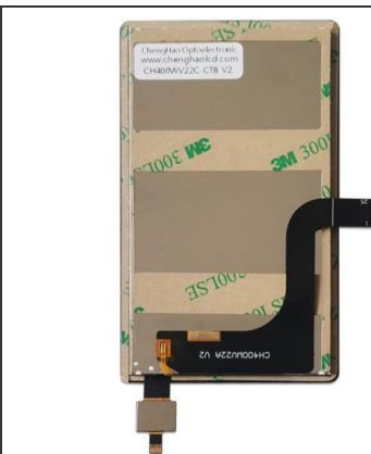
Chenghao Optoelectronic provides extensive customization services, including FPC shape and pin number adjustments, interface modifications (SPI, MCU, RGB, etc.), brightness tuning (300-1500 cd/m<sup>2</sup>), operating temperature adaptation (-45~+90), glass cover customization, anti-glare treatment, and anti-electromagnetic interference solutions, catering to diverse project needs.
