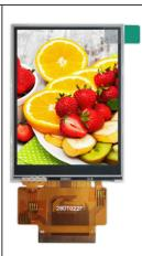
To ensure seamless integration, the CH280QV22F-T supports multiple interface protocols, including SPI, MCU (parallel), and RGB, providing developers with versatile connectivity options. Its compact physical dimensions of 50.0 x 69.2 x 3.4 mm and a 50-pin FPC connector facilitate easy installation in space-constrained designs.
