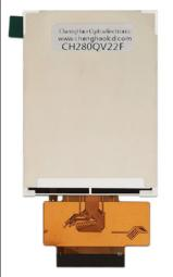
The operating temperature range of CH280QV22F is -20°C to +70°C, while the storage temperature can reach -30°C to +80°C, which enables the module to operate stably in various extreme environments and meet the needs of industrial and consumer electronics. This wide temperature feature makes it very suitable for use in harsh environments, such as factory floors, outdoor equipment, and medical equipment.
