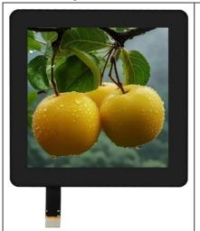
One of the standout features of the CH400WV23A-CTBA is its use of IPS (In-Plane Switching) technology, which provides wide viewing angles of 80 degrees in all directions. This ensures that users can view the display clearly from various positions without experiencing significant color distortion. The module also incorporates a capacitive touch panel, allowing for smooth and responsive interaction, which is essential for modern user interfaces.
