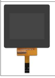
The operating temperature range of the CH200QV03B-L is -  $20^{\circ}$ C to  $70^{\circ}$ C, and the storage temperature range is - $30^{\circ}$ C to  $80^{\circ}$ C, ensuring its stability and reliability under extreme environmental conditions. This makes the module particularly suitable for industrial automation, medical equipment, and other applications that need to work in a changing environment.
