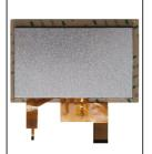
Touch technologyCH700WV03A-CTBA is equipped with a capacitive touch panel and supports multi-touch, allowing users to perform various operations through simple gestures. This touch technology not only enhances the interactive experience, but also makes the operation more intuitive and convenient. The thickness of the touch panel is 0.7mm and has a transmittance of  $\geq$ 87%, ensuring a good display effect.
