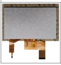
(3) Environmental adaptability CH700WV03A-CTBA has an operating temperature range of -20°C to +70°C and a storage temperature of -30°C to +80°C, making it suitable for industrial control, smart home, medical equipment and other fields. This wide temperature adaptability ensures its reliability in extreme environments and meets the needs of customers in different application scenarios.
