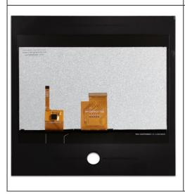
The design of the touch panel not only takes into account the user's operational convenience, but also focuses on durability. The module's touch glass is 1.1 mm thick and has a hardness of 6H, which has good scratch resistance and is suitable for frequently used environments. This feature ensures that the CH700WS02D-CTH can maintain a good user experience in various application scenarios.
