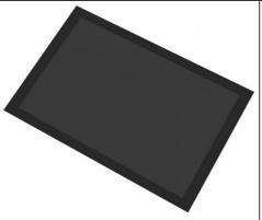
In terms of environmental adaptability, CH101WX05A-CTC performs well. The operating temperature range is -20°C to 70°C, and the storage temperature range is -30°C to 80°C. It can adapt to a variety of harsh environments such as outdoor and industrial. It can operate stably even in the cold northern winter outdoors or in high-temperature industrial plants. Moreover, the product complies with RoHS environmental protection standards and is safe and reliable in material use.
