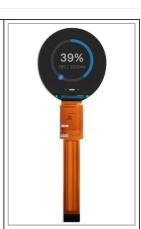
CH132HV01A also supports SPI interface for easy connection with other devices. The module not only supports sample provision, but can also be customized according to customer needs to meet the special requirements of different projects. Its wide range of application areas include industrial control, smart home, medical equipment, instrumentation, artificial intelligence, and Internet of Things devices, showing extremely high flexibility and adaptability.
