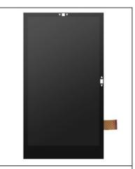
In terms of brightness, the CH550FF01A-CTB has a maximum brightness of up to 600 cd/m², ensuring good readability in different lighting conditions, especially suitable for outdoor use. It is also equipped with a capacitive touch panel and supports multi-touch, which enhances the user interaction experience and makes the operation more intuitive.
