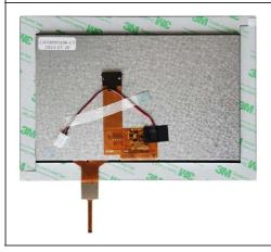
Customers can customize the interface type according to project requirements to ensure compatibility with the control system. In addition, the module has an operating temperature range of -20 to +70°C and a storage temperature of -30 to +80°C, making it suitable for applications in many fields such as industrial control, smart home, and medical equipment.
