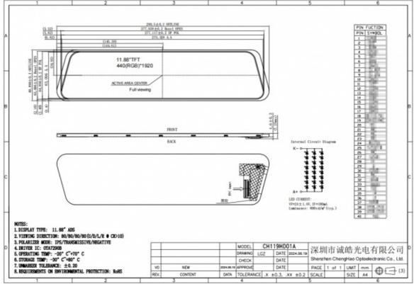
This Sunlight Readable display is an IPS LCD screen module that uses a Module Interface of MIPI. It has a resolution of 440x1920 Dots and a Luminance of 800 Cd/m2. The display can operate within a temperature range of  $-20 \sim +70$  °C and can be stored at temperatures ranging from  $-30 \sim +80$  °C. It has a viewing direction of 80/80/80/80 and a color depth of 16.7M. The FPC Pin Number is 40pins and it has a backlight consisting of 24 Pcs White LED.
