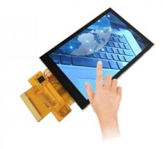
Chenghao Optoelectronic CH350HV37A-CTC is a 3.5 inch small touch tft lcd display module, which includes a tft lcd panel, a touch panel, a driver IC, an FPC and a backlight component.
