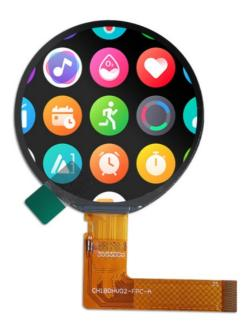
ChengHao Display Model CH180HV02A Overview ChengHao Display model CH180HV02A is a color active matrix thin film transistor (TFT) liquid crystal display (LCD) that uses amorphous silicon TFT as a switching device. This model is composed of a TFT LCD panel, a driving IC, a high brightness back-light, a capacitive touch panel and FPC.
