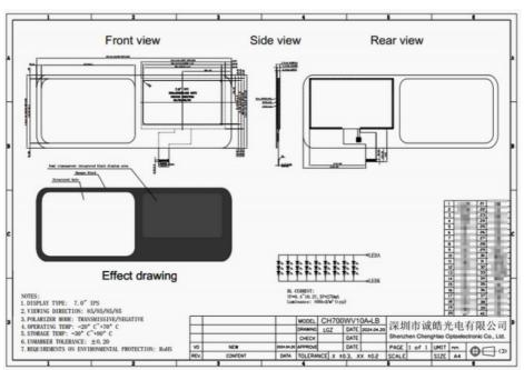
The CH700WV10A-LB module is designed to function effortlessly in extreme environmental conditions. Operating within a range of -20°C to +70°C and a storage temperature range of -30°C to +80°C, the module can withstand a broad range of temperatures. This makes it suitable for a wide range of applications requiring a reliable display solution.
