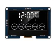
This is a 2.42-inch OLED display module with a resolution of 128x64 and supports smooth operation in environments as low as -40°C and as high as +70°C.
