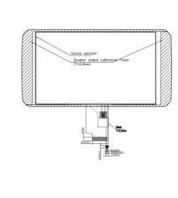
Product Name: TFT Display Module Module No: CH700WS02D-CTG Lcd Type: 7" IPS TFT+CTP Display Mode: IPS/Transmissive/Normally Black Number of dots: 1024\*3(RHB)\*600 Viewing Direction: 80/80/80/80 TP Type: CTP TP Interface: I2C Outline Size: 205.32\*106.45\*8.23 mm Active Area: 154.2144\*85.92 mm Operating Temp: -20~ +70°C Storage Temp: -30~ +80°C BL Current: VF=8.4~10.2 V,IF=300 mA Backlight Brightness= 1000 cd/m2
