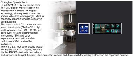
interaction. Support 3 line SPI+24 bit RGB multi-interface to communicate with the outside world. If this square color LCD touch screen does not meet your project needs, we have many similar display solutions available to
