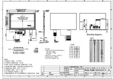
1. 5 inch tft lcd 800x480 Capacitive touch dispaly RGB Interface
